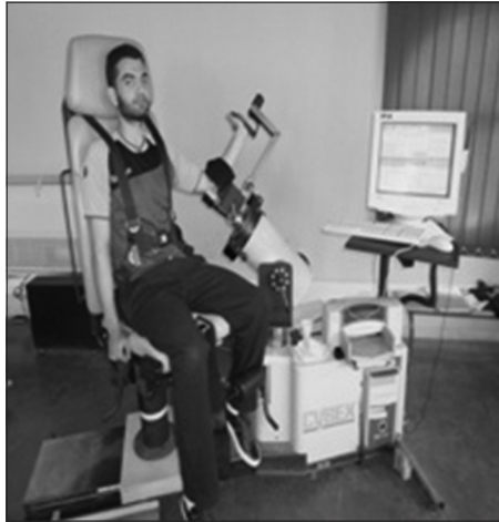
Figure 1: Isokinetic testing set-up for internal and external rotators muscle of the shoulder with the Cybex dynamometer.
